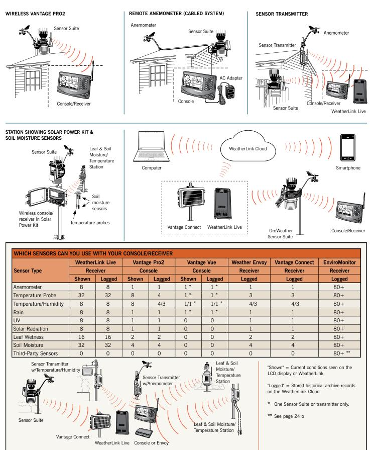
Each WeatherLink Live, Vantage Pro2, Weather Envoy and Vantage Connect console can receive data from up to eight different transmitting stations.
