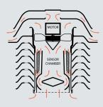
3. Choose a model with 24-Hour Fan-Aspirated Radiation Shield
